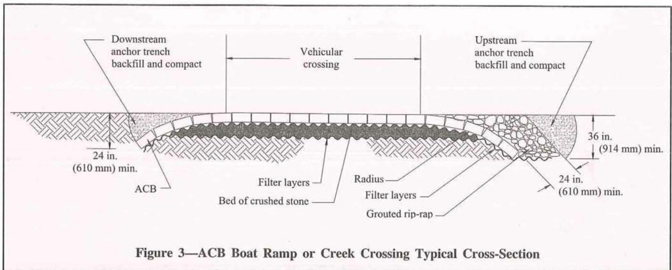
Figure 3—ACB Boat Ramp or Creek Crossing Typical Cross-Section
