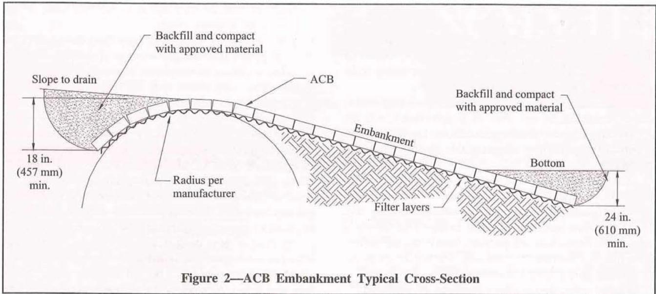
Figure 2—ACB Embankment Typical Cross-Section
