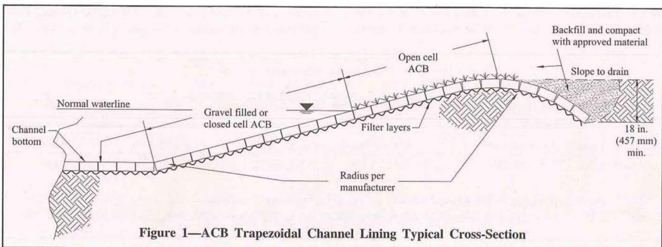
Figure 1—ACB Trapezoidal Channel Lining Typical Cross-Section
